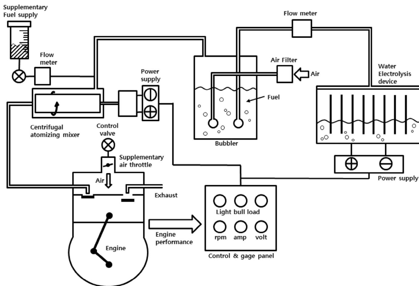
Fig. 1. Experimental layout for the generation of vaporized gasoline and WEG mixture fuel and a burning system with a single cylinder engine.
